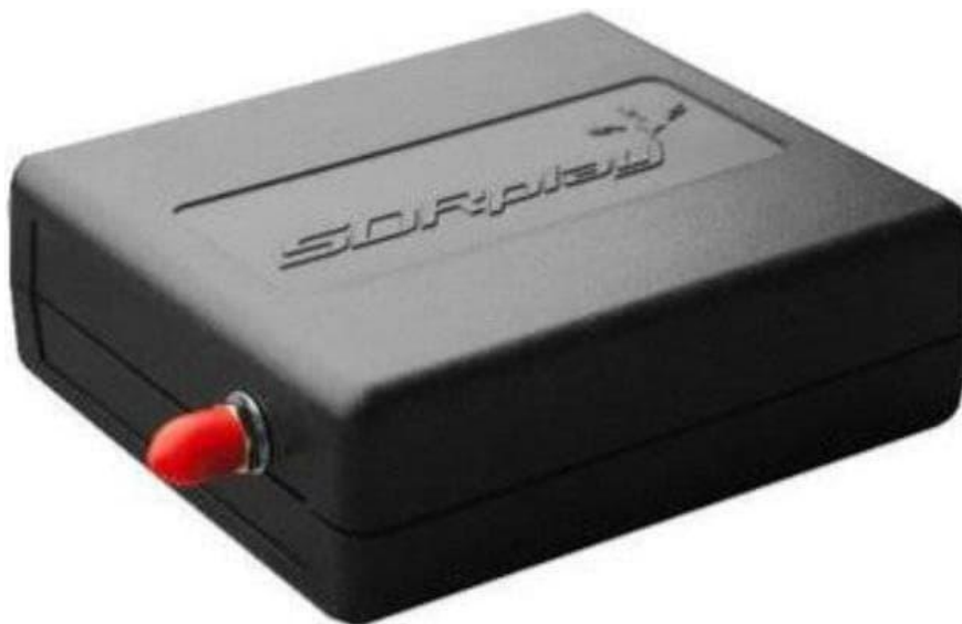
Fig. 8: Typical software defined radio (SDR). There are many other, similar devices which allow to receiver frequencies up to 1420 MHz and to provide analog-digital converted data via USB-cable to a computer for further data analysis. I tested many other (cheaper) SDRs in form a a USB-stick. But data quality proved to be best with this SDRplay.
