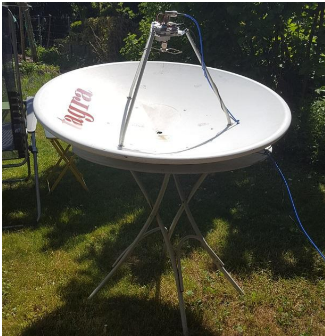
Fig. 1: Old, used parabolic dish from flea-market which I got for 100$ several years ago. Unfortunately, I don't have access to a mounting- and tracking-system. Therefore the dish was put on a garden table and tilted with some wooden blocks underneath, such that the antenna beam is pointing to a dedicated position on the sky.
