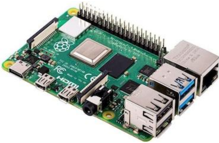
Fig. 9: Typical Raspberry Pi as backend for the radio telescope. In my case I use both ways to communicate with Raspberry.
